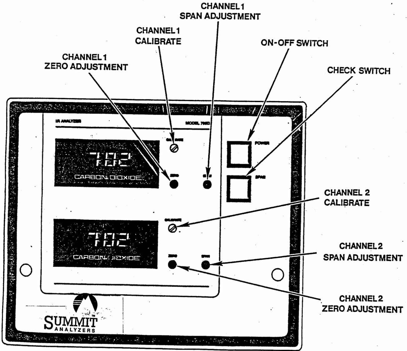
Figure 5: IR-702 Front Panel
