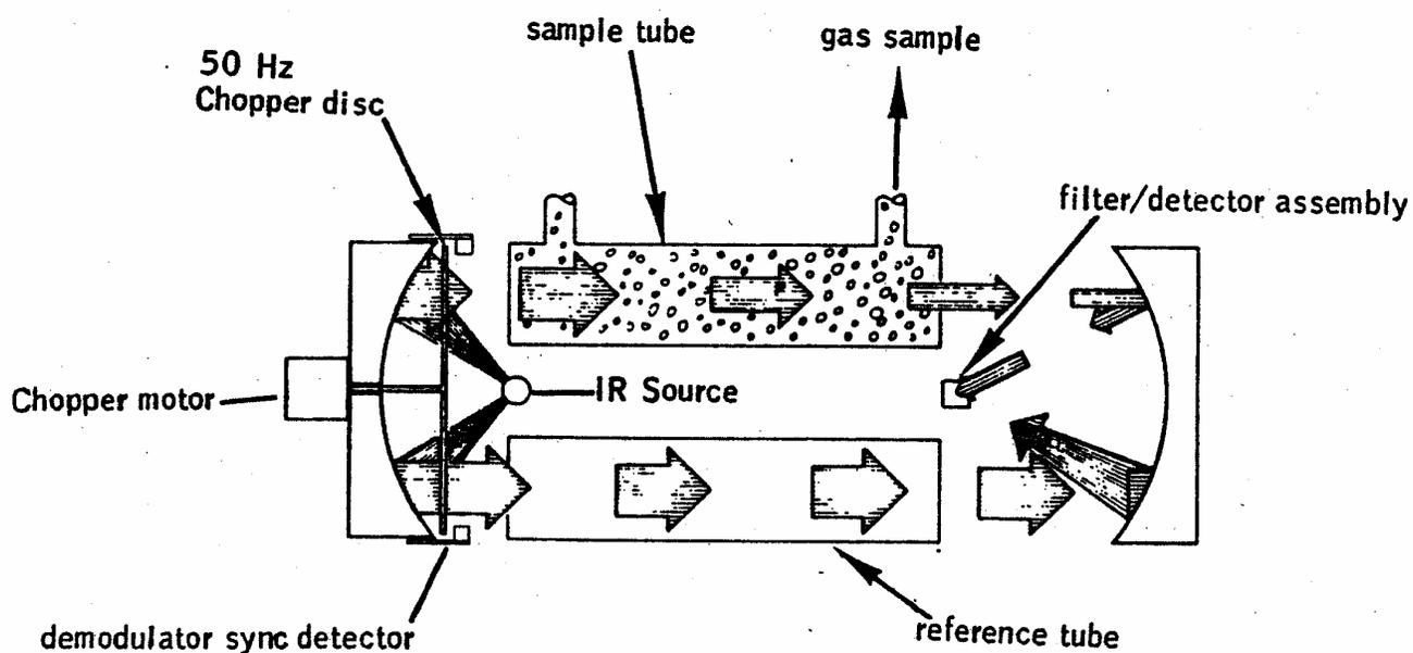
Figure 6: Optical Bench Schematic
