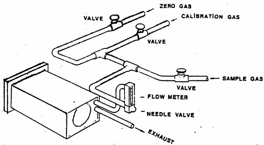
Figure 4: Typical Gas Handling System
