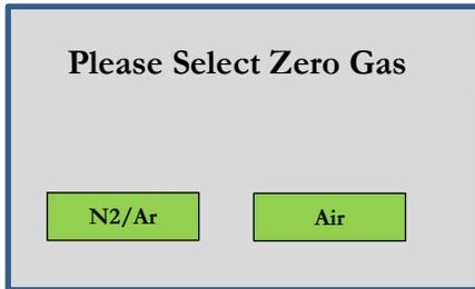
By pressing the **Calibration** button from the main settings screen the analyzer goes into standby and prompts for the type of purge gas. The options are Nitrogen, Argon and Air. Zero gas should flow through the unit while zero is performed.
