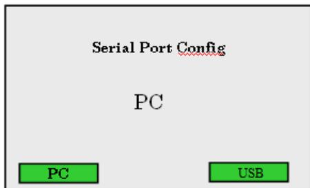
This selection defines the communications on the serial port. Select PC if remote control and display is desired. Select USB for the optional USB data collection.
