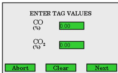
Once the "zeroing" has completed you will see this screen. Enter each gas tag value by pressing the corresponding box.
