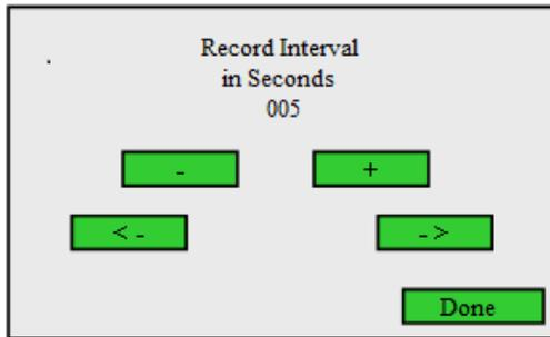
When the optional USB data collection is configured in the analyzer the Data Recording screen sets the interval used to record data readings. If the interval is set to zero no data recording occurs.
