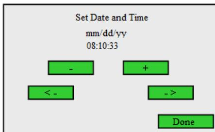
Use the plus and minus buttons to change the value in the highlighted field. Use the left and right arrows to move between fields. When finished press Done to return to the Measurement Mode window.
