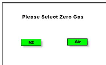
The options are Nitrogen, Argon or Air. Once the zero gas is selected the analyzer will start the zero process and displays:
