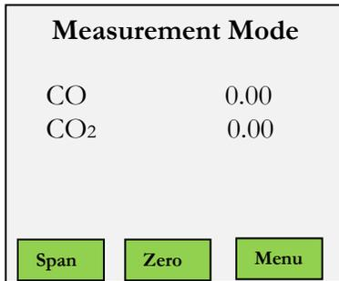
The Measurement Mode Screen is referred to as the **Home Screen**. From this screen you can access the Configuration Menu by touching the MENU button.
