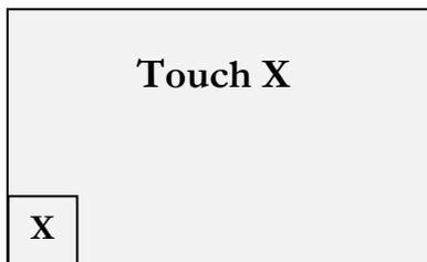
LCD Touch Screen Calibration; follow the instructions on the screen. Touch the X on the lower left side, then on the upper right side.
