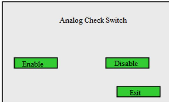
This feature will send full voltage out all analog ports when Enable is selected. The voltage will stay at full range until Disable is selected. When exiting this screen the switch will be set to disabled.
