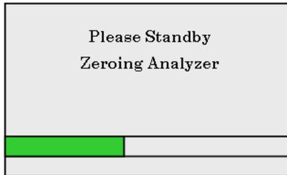
The analyzer goes into standby and begins to purge the gas lines. The bar at the bottom of the screen shows the progress of the process as it moves from left to right.
