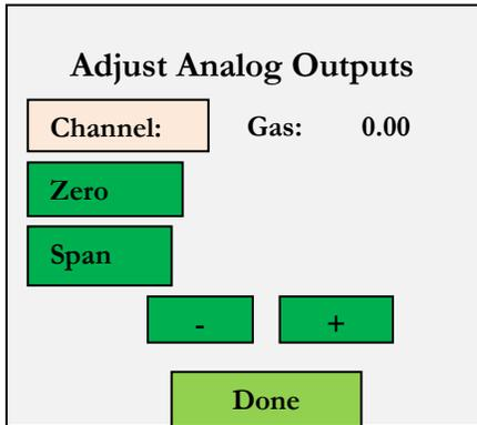
From the Home Screen select **Adjust Analog Outputs**. For each gas measured configure the low (zero) and high (span) by pressing the value in the box. Use - and + increment/decrement to set the corresponding option.
